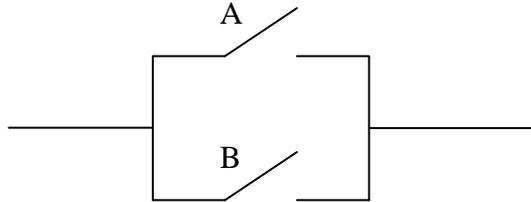
It is a parallel circuit, and at least one switch must be closed (on) for the circuit to be complete from left to right. You can see, then, that this is the same as “A or B”, since “A or B” is true when either A is true or B is true or both.
