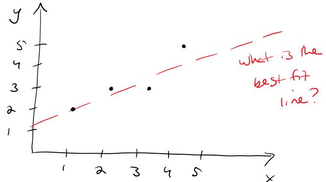
$$\left\{ \begin{array}{l} y_1 = mx_1 + b \\ y_2 = mx_2 + b \\ y_3 = mx_3 + b \\ y_4 = mx_4 + b \\ \vec{y} = m\vec{x} + b \end{array} \right.$$
